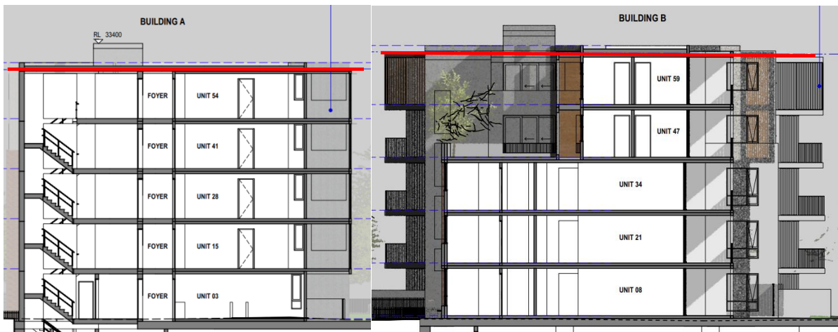
Figure 3: Extract of the cross sections of Buildings A (left) and B (right) within the proposed development. The 15-metre height plane is denoted by the red lines.
