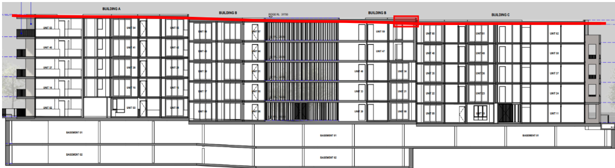
Figure 2: An extract of the long (i.e. east-to-west) section plan of the proposed development; the 15-metre height plane is denoted by the red line. The tallest point of the building that does not include lift overruns is denoted by the red box.
